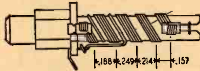
Fig. 9—Permeability tuner used by Zenith.
